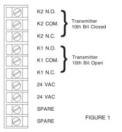
Back the screws on the terminal block off slightly and insert your wiring lugs (or wire) under the appropriate set screw.
