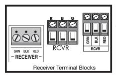
**Step 1:** The RB709U-NB will replace the gate opener receiver; disconnect the gate opener receiver's RED, BLACK, and GREEN wires from the receiver terminals on the gate opener control board.
