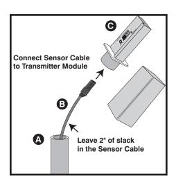
**Step 5:** Run the Sensor Cable **(B)** through the Mounting Post **(A)** and plug it into the connector at the bottom of the Transmitter Module **(C)**. Allow 2 in. slack in the cable to prevent damage to the connector if Transmitter Module is removed.
