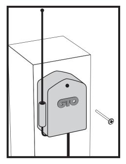
Step 3: Connect the RED and BLACK wires from the Receiver to the power supply (see illustration, page 5).
