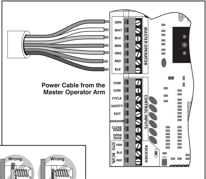
**NEVER SPLICE WIRES** Splicing permits corrosion and seriously degrades the wire's ability to carry an adequate current.
