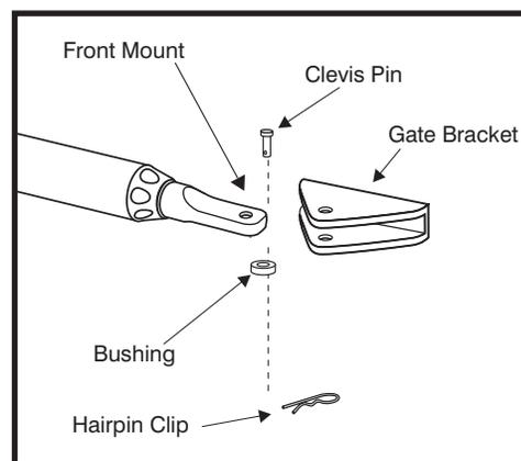
NOTE: Substitute a Pin Lock
