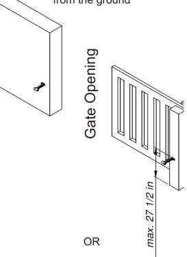
Install contact sensor on the leading edge of the gate and all other identified pinch-points
